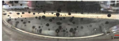
Figure 7. Suspended microspheres (black dots) printed inside the mineral oil.
